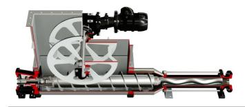
This model features a rectangular hopper, joint protection sleeve and an enlarged auger feed screw to move the product to the hydraulic part. A "B" Module is installed on the hopper which feeds the screw by means of a wheel device to prevent bridging. Suitable for pumping non-flowing materials with up to 40% solids content prone to bridging and plasticizing.
