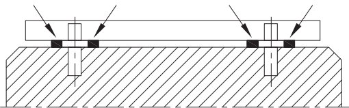
Fig. 2. Foundation, baseplate and fitting the shims
