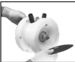
6.1.20 Remove the first diaphragm
