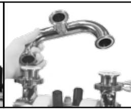
6.1.15 Position the gaskets and the suction manifold.
