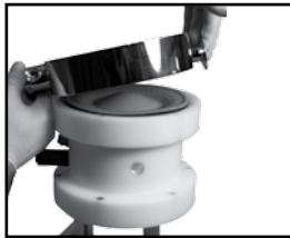
6.1.16 Remove the pump bodies
